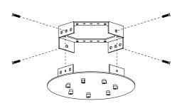
Secure canopy to mounting bracket using the provided screws. Route pigtails to one of the open sides of the mounting bracket.
